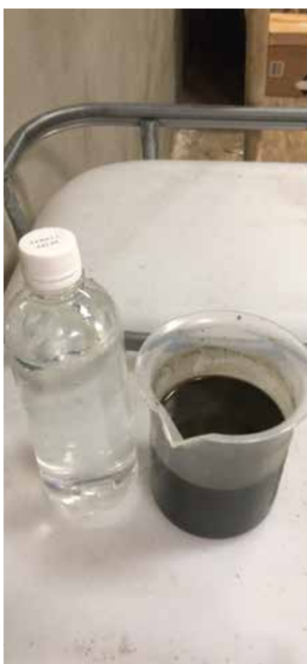
Figure 4. Raw slurry before (dark) and after (clear) a single pass through the vibrating RO pass
