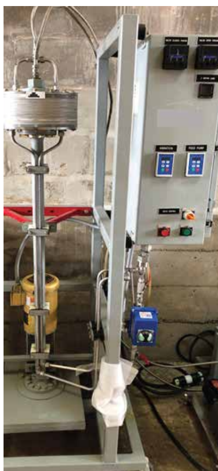
Figure 3. Detail of vibrating RO for the single pass treatment of raw slurry
