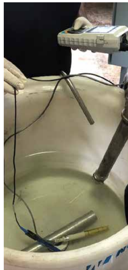
Figure 5. Measuring the conductivity of the permeate (clear water)
